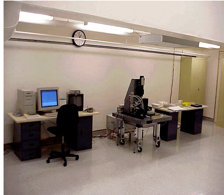
Strips assembly area showing vision assisted alignment station
