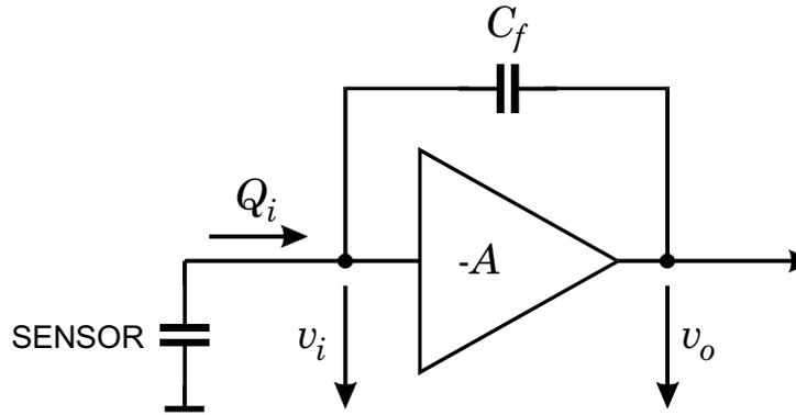
FIGURE 5. Basic configuration of a charge-sensitive amplifier
