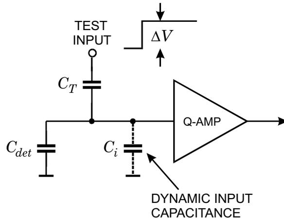
FIGURE 6. Charge calibration circuitry of a charge-sensitive amplifier
