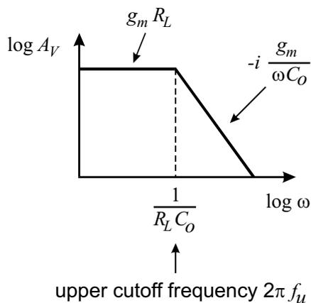
**FIGURE 9.** Frequency Response of a simple amplifier
