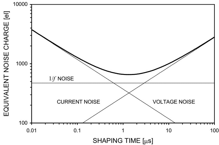
**FIGURE 18.** Equivalent noise charge vs. shaping time
