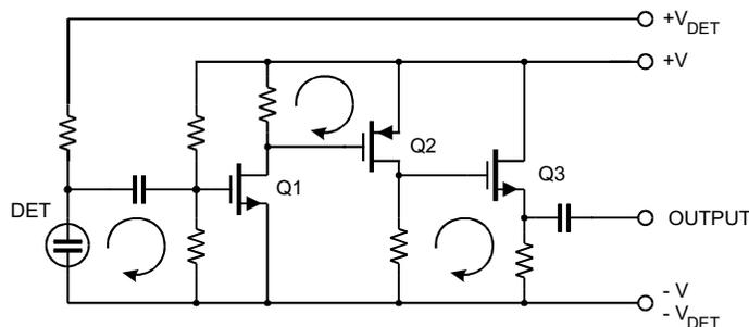
**FIGURE 23.** Local signal current return paths in a sensor and amplifier.
