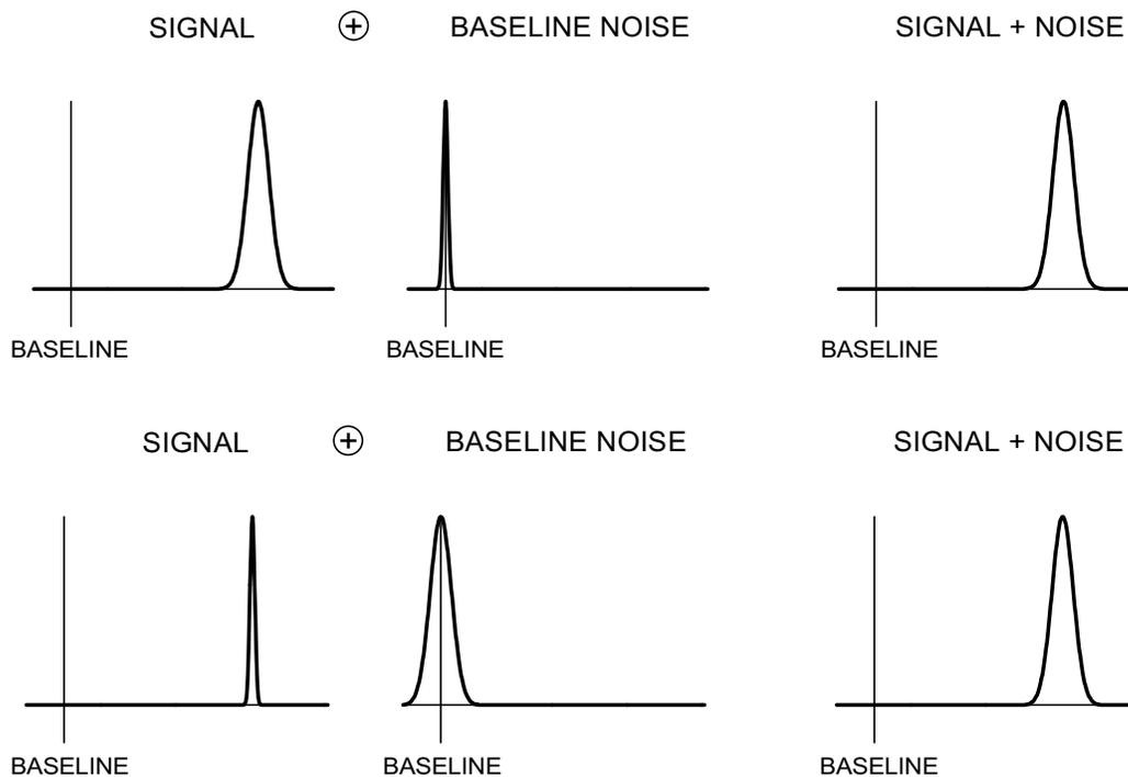
**FIGURE 12.** Signal and baseline fluctuations for large signal variance (top), as in scintillation detectors or proportional chambers, and for small signal variance, but large baseline fluctuations, as in semiconductor detectors or liquid Ar ionization chambers, for example.
