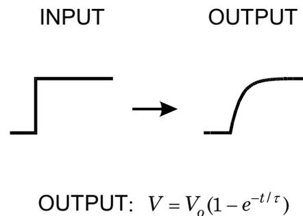
**FIGURE 10.** Pulse response of a simple amplifier
