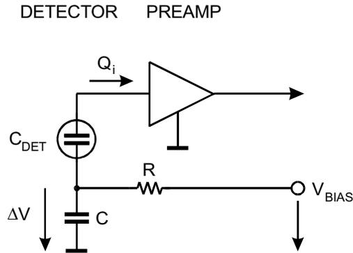
**FIGURE 21.** Spurious charge injection through the sensor.
