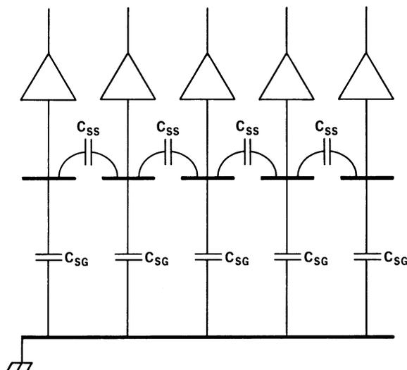
FIGURE 11. Cross coupling in a silicon strip sensor
