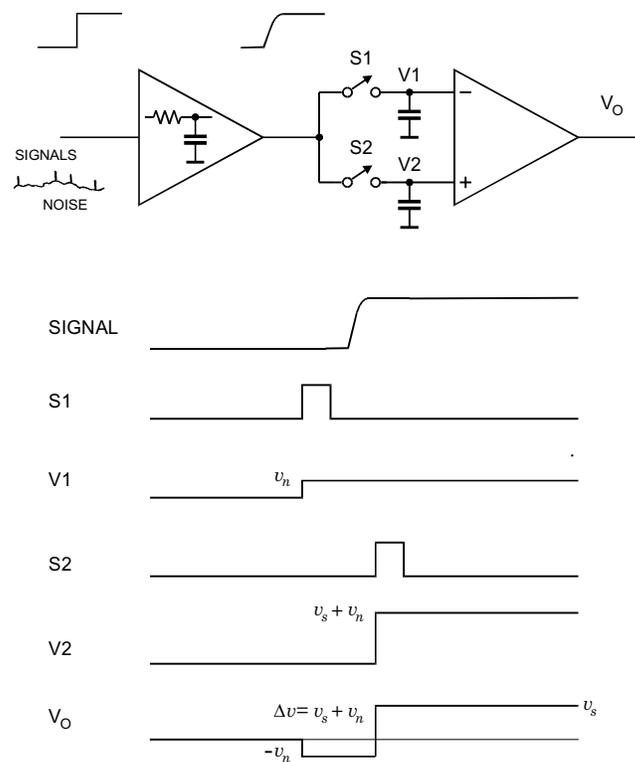
**FIGURE 20.** Principle of a correlated double sample shaper
