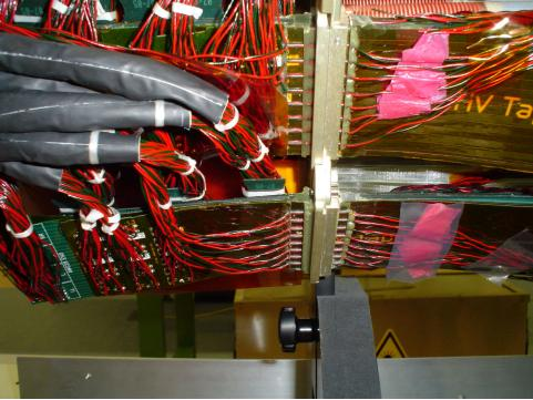
ISP flange bolts removed and flange dropped about inch. Slide back OSP. Epoxy flash. Removed. Put back flanges. OK. Lift up and insert into BPSS! The corner nearest center of ISP A2 is not properly notched and the slot in the tab is not full width. This made this go up by about 1mm, could not engage screw – see below.
