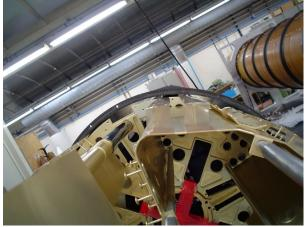
The two cans are mounted on the top. Pushed BPSS through. No weight on cans. Passed through without touching but visual clearance tight in some spots. Decided to use shims to get rough measure of clearance. All measurements are orientation looking into shell from BPSS out side that is from the right into the shell as shown in first picture in this log. Measure clearance to buttons.
