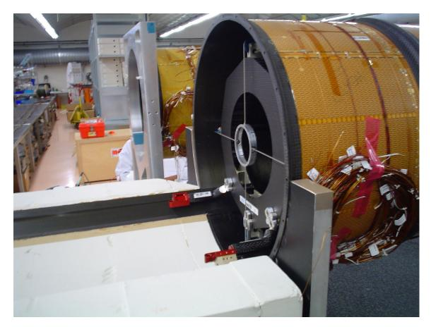
We did a number of measurements to understand if the BPSS structure is centered in the PST. Measurements to the longerons, blocks on the longerons, etc. It appears that BPSS is off center to roughly the left by about 1mm. Top to bottom comparisons are hard because it's hard to measure on the bottom with what we have. Getting tired. Need to do a consistent set of measurements next.
