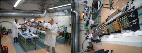
Continuity testing held up because fibers in the service panel slots are in the way of getting at bolt head at two of three spots. The fiber folks worked on this but it's a pain. Need to think about revised sequence.
