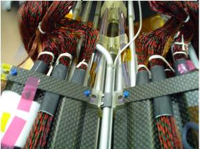
The holes in the SLA on the SQP were opened up slightly. Some filing of the PP0 boards and around the button heads on the BPSS. Put A3-4 back up to BPSS and finally made it fit. Since loading is not vertical wants to slide down just a bit making easy engagement of bolts on SLA at bottom hard. But still we managed to tighten all but one and could engage that one.
