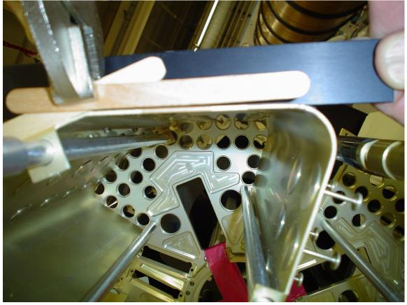
The buttons to the left in this picture are higher on the left face in this picture than the right face. This seems to explain part of the clearance difference.
