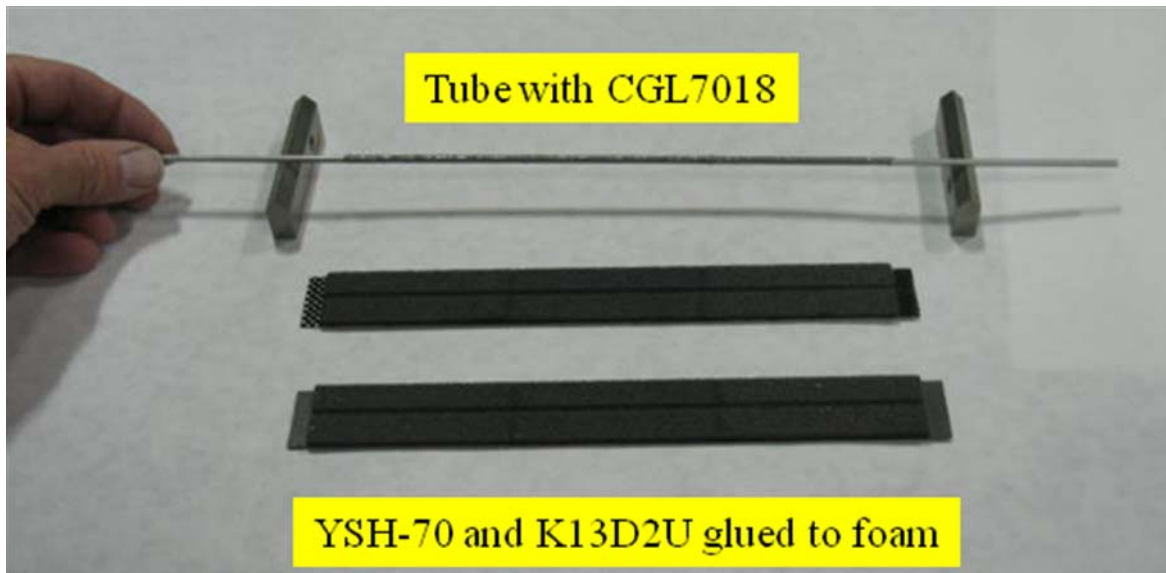
Figure 2 Principal components of first foam prototype structure described in the text.
