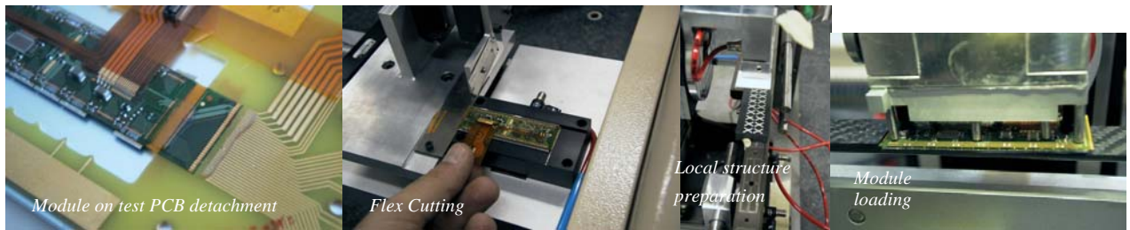
Figure 12 Task sequence of module assembly on ATLAS pixel detector.
