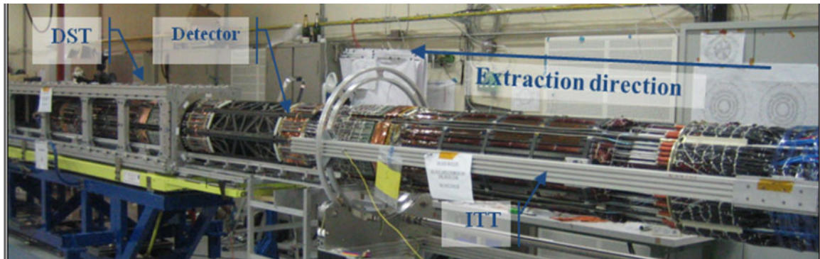
Figure 7.7.1 The pixel detector leaves the tool on which has been integrated (ITT) and it enters into the transportation tool [DST]. The blue structure underneath is equipped with pivoting and spring loaded wheels for an easy and shock free transfer outside the building.
