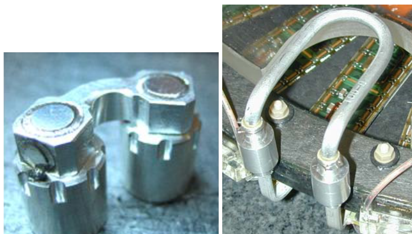
Figure 8.4.13 (a) U-link structure used to connect to staves to form a bi-stave unit and (b) U-tube for connecting disk sectors, during assembly of a disk.
