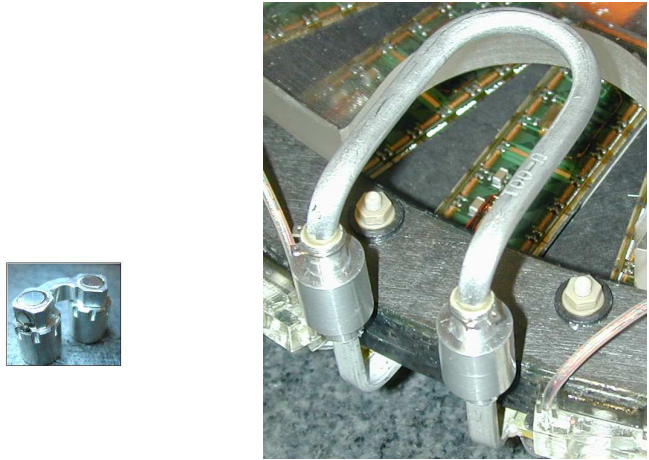
Figure 32. (a) U-link structure used to connect to staves to form a bi-stave unit and (b) U-tube for connecting disk sectors, during assembly of a disk.
