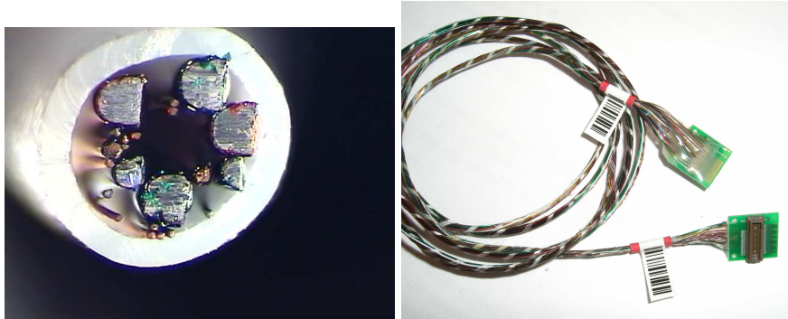
Figure 23. (a) Section through a disk T0 cable and (b) detail of a barrel T0 cable.
