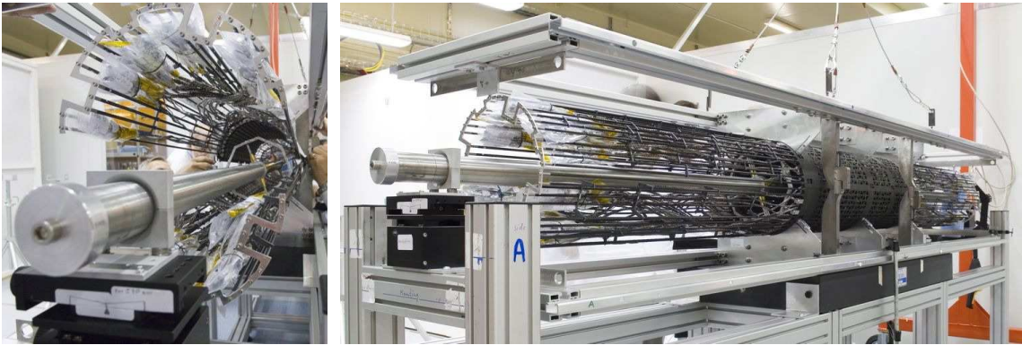
Figure 12. Clamping of the Layer 2 half-shells. The top half is craned onto the bottom one resting on the STT (see text). The picture shows the mechanism that guides the process. The stainless steel pipe, visible along the the axis of the shell, was used to guide the insertion into the global frame and was removed afterward.
