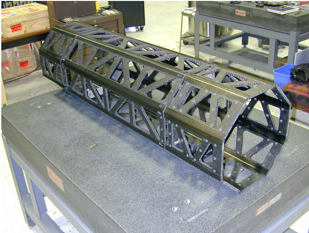
Figure 2. The support frame for the pixel detector.
