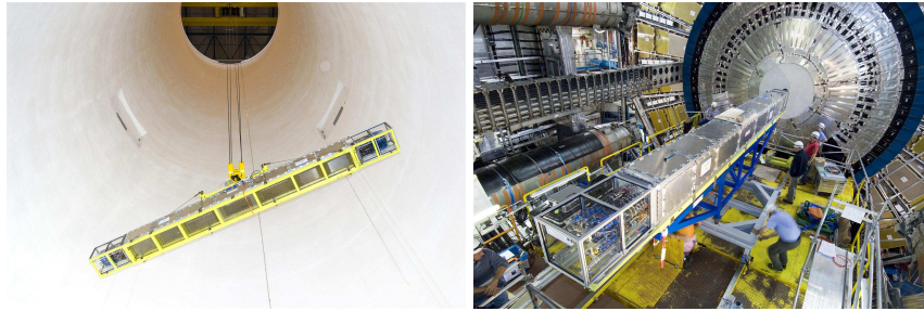
Figure 49. (a) the pixel detector in the Dummy Support Tube (see text) being lowered into the ATLAS underground hall and (b) the Dummy Support Tube and pixel detector on a platform between the Inner Detector area and the endcap calorimeter.
