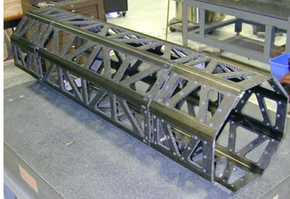
Figure 7.1.2 The support frame for the pixel detector.
