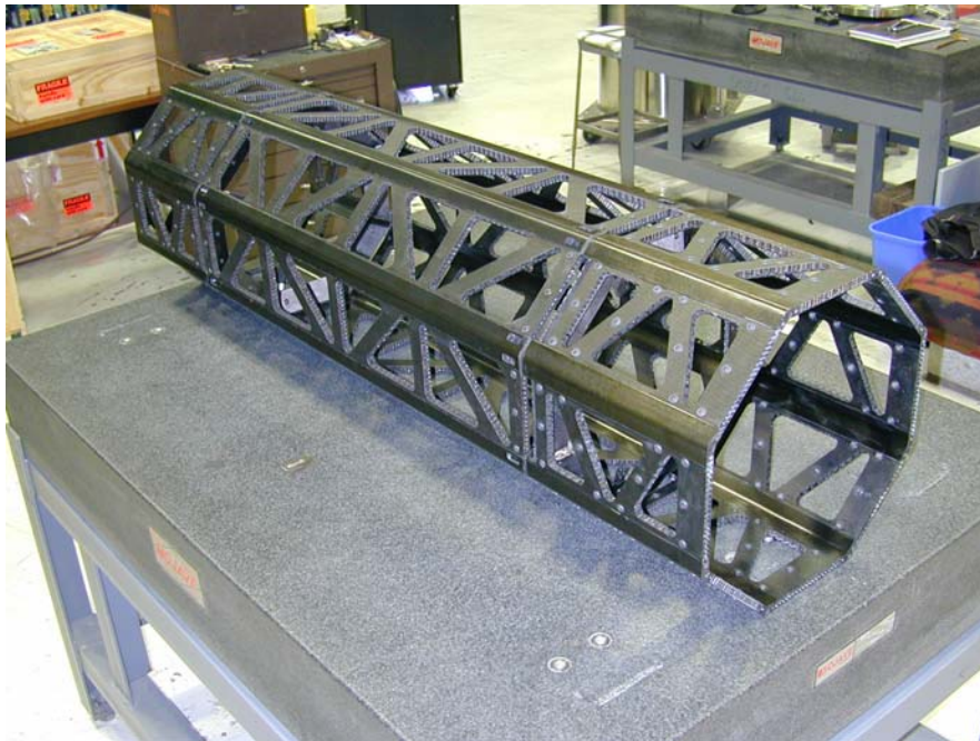
Figure 2: The support frame for the pixel detector.
