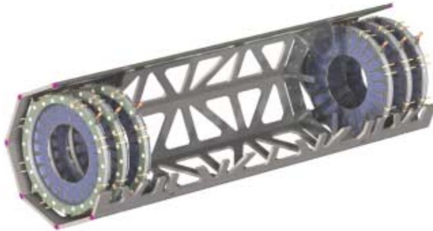
Figure 1. ATLAS Pixel disk structures(support rings and disk sectors) inside the global support frame.
