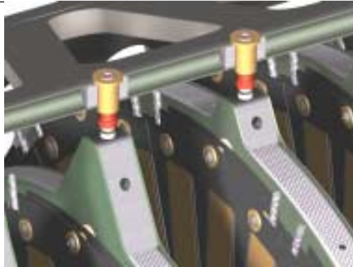
Figure 3. PEEK based adjustable radial mount for the disk support ring. View rotated 45° for convenience of display.
