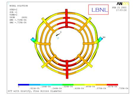
Displacements without Pixel Detector,  $max = 74 \ \mu M$
