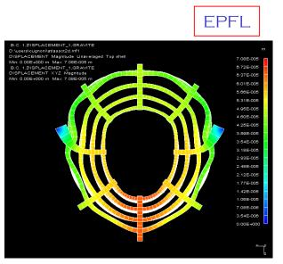
Displacements without Pixel Detector,  $max = 70 \ \mu M$
