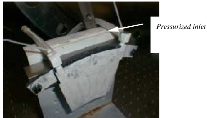
Figure 25. Photograph of HYTEC sector pressure test setup. Inlet tube at upper right is open to pressure source. Exit tube at the left is sealed to prevent flow during the test.
