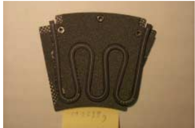
Figure 5. Anodized tube in foam showing construction.
