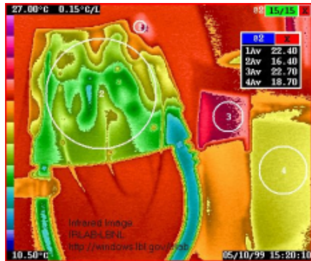
Figure 7. Infrared image of aluminum-tube prototype #4 at 48W of power with 10 cc/sec flow of coolant.
