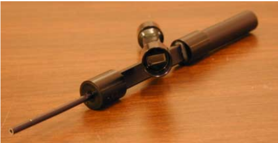
Figure 31. Test piece showing square-to-round transition from sector cooling to other cooling connections.
