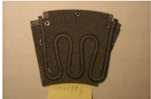
Figure 5. Anodized tube in foam showing construction.
