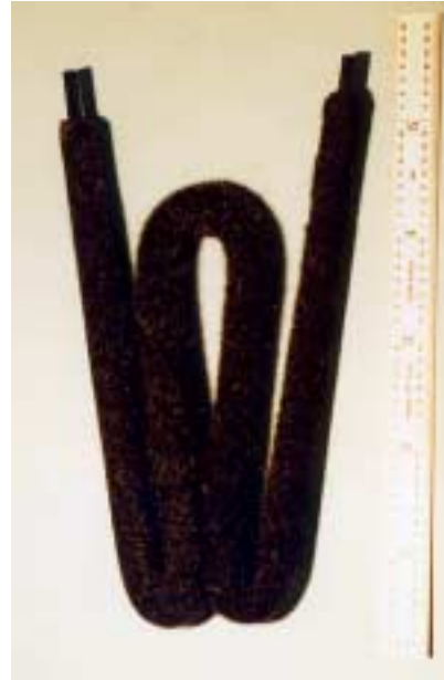
Figure 2. Glassy carbon tube with fibers attached.
