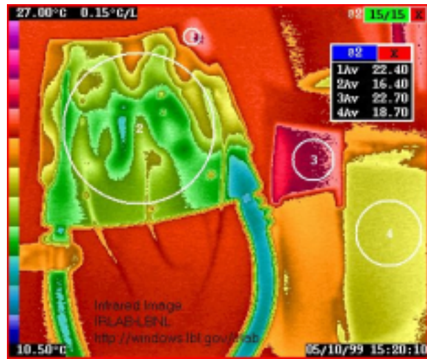
Figure 7. Infrared image of aluminum-tube prototype #4 at 48W of power with 10 cc/sec flow of coolant.
