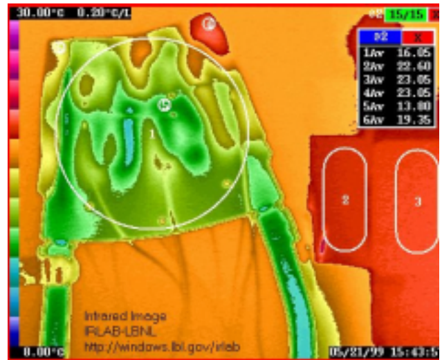
Figure 13. Aluminum-tube prototype #4 after pressure cycling (see text).
