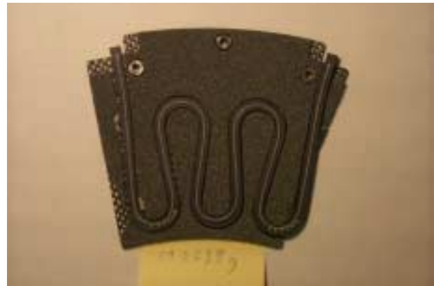
Figure 5. Tube in foam showing construction.
