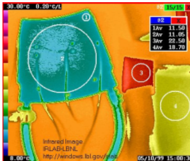
Figure 6. Infrared image of aluminum-tube prototype# 4 without power at 10 cc/sec flow of coolant.
