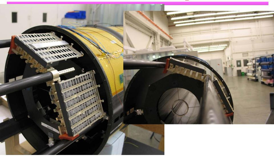
Shim backbone to bring clearance between outside of longeron on backbone to shell of about 15.5mm 2 M. Gilchriese
