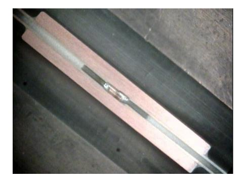
Lessons learned, Limit solder to exact amount needed, exact precision at all steps of sleeve manufacture, Address flux intrusion, heat control.
