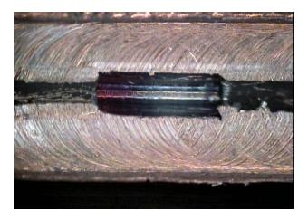
After wet sanding and acid etch, This is what could be seen. Note darkened cap. tube on the left (flux).
