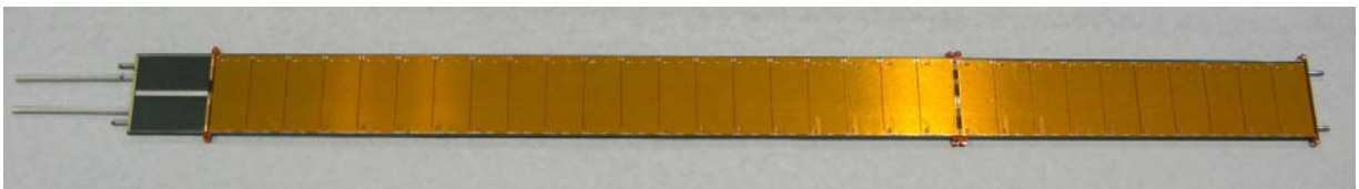
Figure 8 Photograph of a prototype stave (about 1 m long) with bus-cables attached (to both sides of the stave). The silver strip seen on the left is conducting epoxy to allow for a connection to be made from the end-of-stave card to the facing of the stave. The bus-cable was made in two parts for this prototype.
