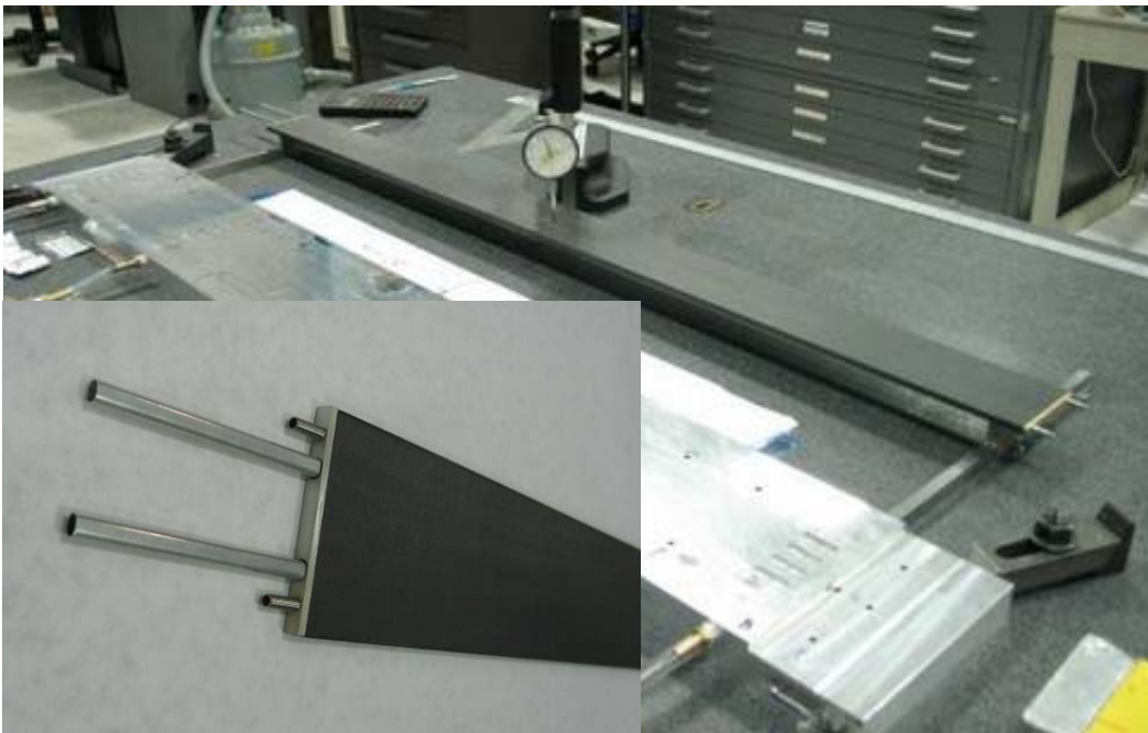
Figure 7 Prototype #3 during deflection measurements. The inset shows the detail at one end of the stave.
