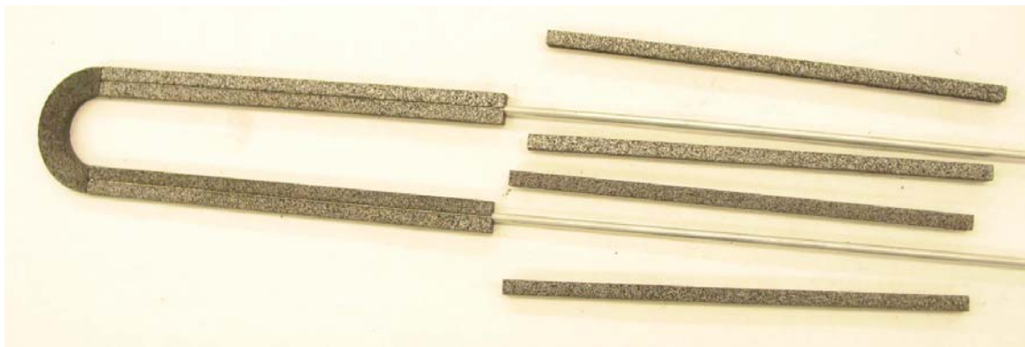
Figure 6 Aluminum pipe (2.8 mm OD) surround by POCO foam pieces, prior to gluing pieces to the tube.
