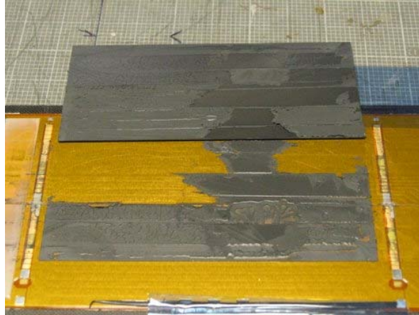
Figure 13 Photograph of a dummy silicon detector glued with SE4445 just after removal of the dummy detector but before clean up of the bus cable areas.
