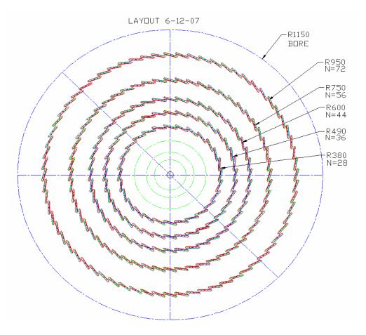
The number of 1m staves is 2x(28+36+44)=216. The number of 2m staves is 2x(56+72)=256. The approximate total area is then  $.105x(216+2x256)=76 \text{ m}^2$ . The disk area is taken as  $23\text{m}^2$ , which is based on the area from "strawman layout 7" times a factor of 1.1 for overlaps. Thus the total area is roughly  $100\text{m}^2$ . We take a wastage factor of about 1.2, which yields a total area of about  $120\text{m}^2$ .
