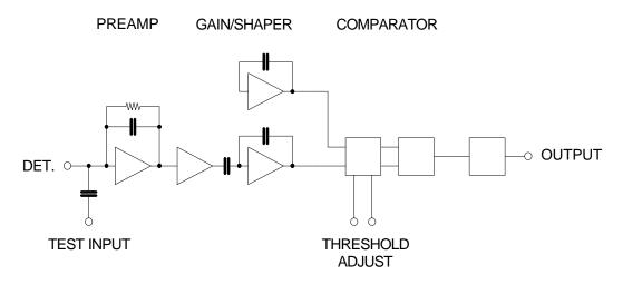
FIGURE 9. Block diagram of a readout channel for strip detectors.
