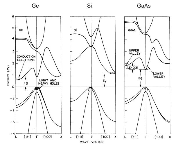
Band Structure in Ge, Si and GaAs vs. Wavevector and Orientation
