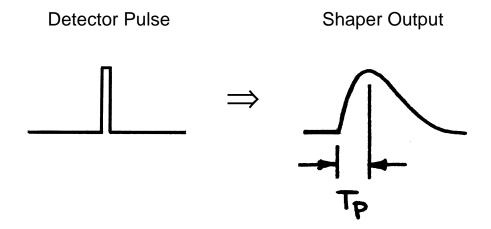
If the shape of the pulse does not change with signal level, the peak amplitude is also a measure of the energy, so one often speaks of pulse-height measurements or pulse height analysis. The pulse height spectrum is the energy spectrum.
