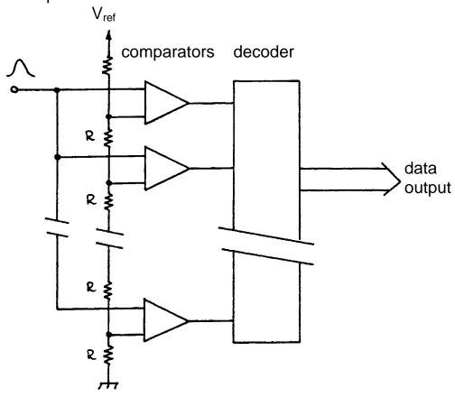
The input signal is applied to n comparators in parallel. The switching thresholds are set by a resistor chain, such that the voltage difference between individual taps is equal to the desired measurement resolution.
