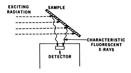
The incident radiation can be broad-band, as long as it contains components of higher energy than the atomic transitions of the atoms to be detected.
