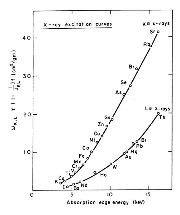
Note the increase in cross section with energy. Using the smallest possible excitation energy for a specific element reduces background from higher energy transitions.
