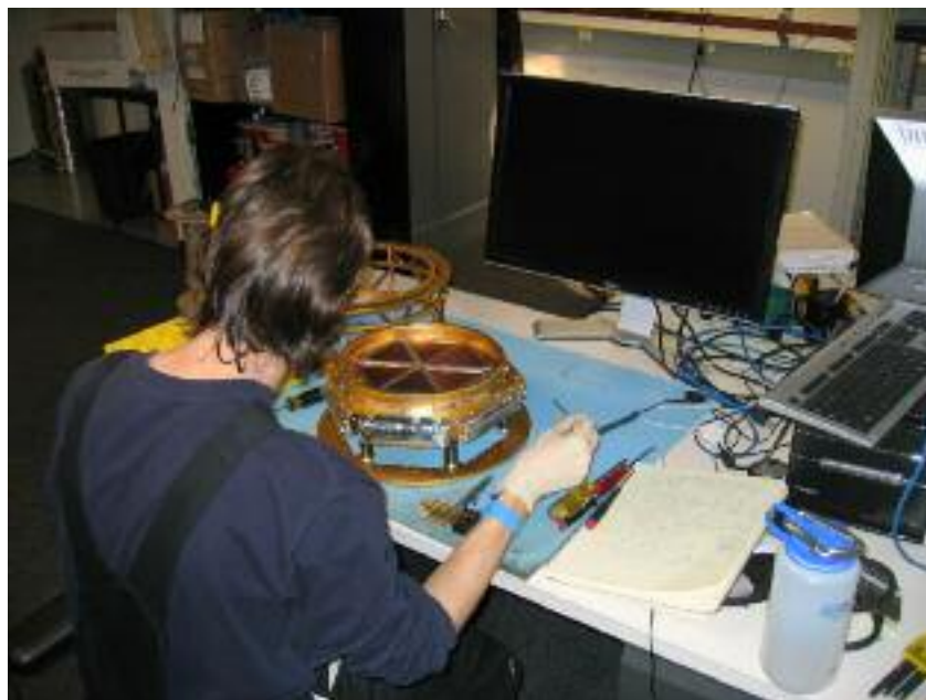
Disassembled focal plane for upgrades
