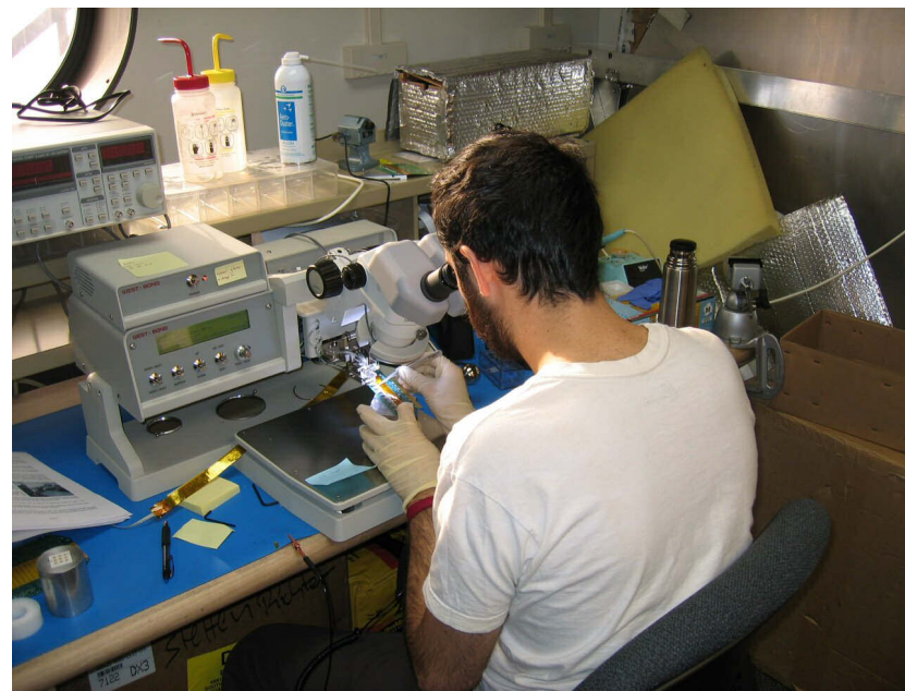
Wirebonding replacement SQUIDs
